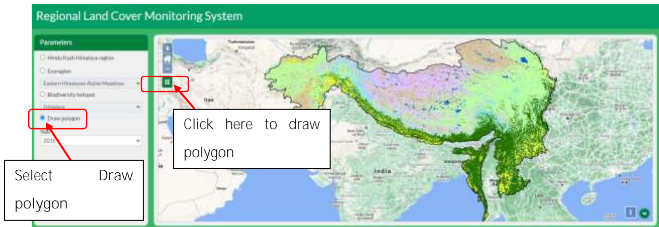
Figure 3 The RLCMS offers a “Draw polygon” feature that allows users to draw a polygon to supply an area of interest After a user completes drawing a polygon on the map window, the Compute button appears just below the “Draw polygon” radio button. (Figure 5). The land cover data for the selected polygon is automatically updated by clicking the Compute button (Figure 7).
